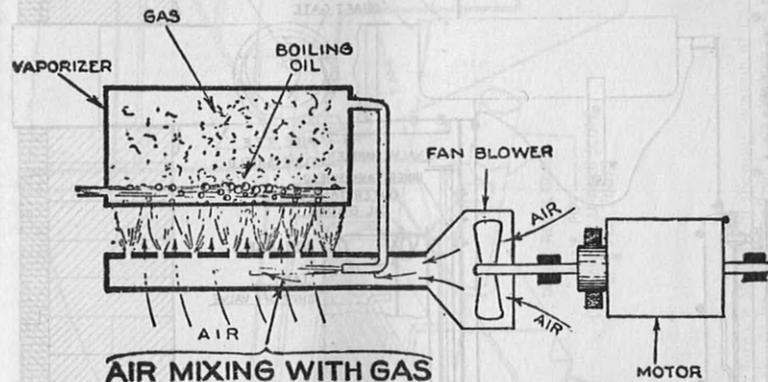
FIG. 3—Elementary gravity feed forced draught *mixing* under flame vaporizing burner.
