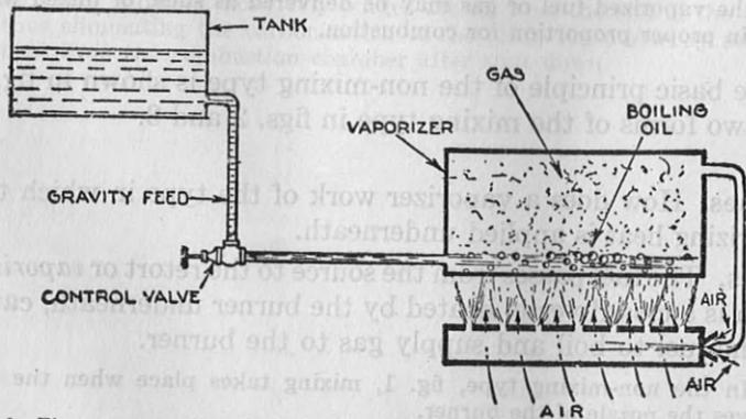
FIG. 2—Elementary gravity feed induction *mixing* under flame vaporizing burner. In this type the vapor issuing from the nozzle draws in air into a mixing chamber where the vapor and air mix, the combustible mixture thus formed passes out through numerous small openings and ignites at the top.
