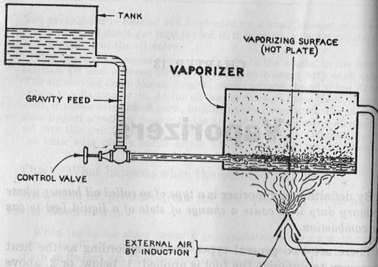
FIG. 1—Elementary gravity feed induction *non-mixing* under flame vaporizing burner. The heat from the flame vaporizes the liquid fuel in the retort. The vapor issuing from the nozzle mixes with the air externally by induction.
